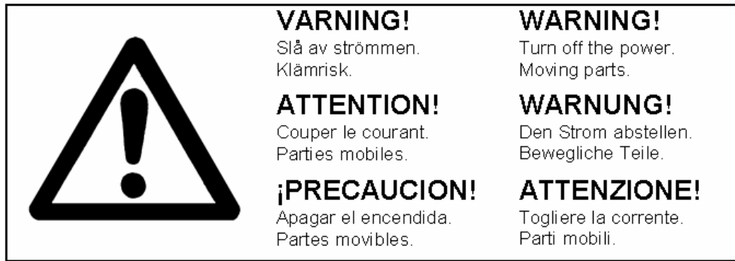
Fig. 4: Warning signs on front hatch
